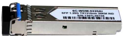
1000Base-BX WDM Singlemode (TX 1310 nm – RX 1550 nm)
