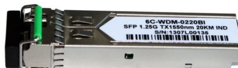
1000Base-BX WDM Singlemode (TX 1550 nm – RX 1310 nm)
