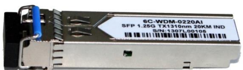
1000Base-BX WDM Singlemode (TX 1310 nm – RX 1550 nm)
