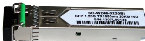
1000Base-BX WDM Singlemode (TX 1550 nm – RX 1310 nm)
